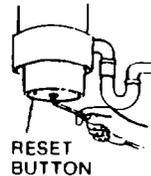
Your Jam Breaker Wrench will free virtually every jam that may occur due to foreign objects entering the disposer. Occasionally, a piece of metal (bobby pin, thumb tack, paper clip, silverware, etc.) causes a jammed condition too tight for your Wrench to handle. To free this type of jam, a pry bar or tool must be used. Do not hammer on pry bar.
