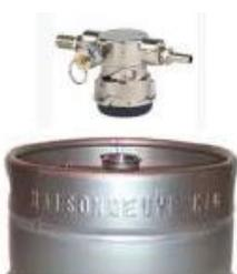
1. Align lug locks on coupler with lug housing in top of keg; insert coupler.
