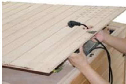
FIG 17 Slip the power cord through Roof Cover
