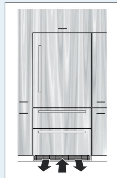
The appliance do not require ventilation considerations in the cabinetry. The required airflow is directed through the toe kick base. It is important to use the provided cover grille for the ventilation opening. This opening must not be covered.
