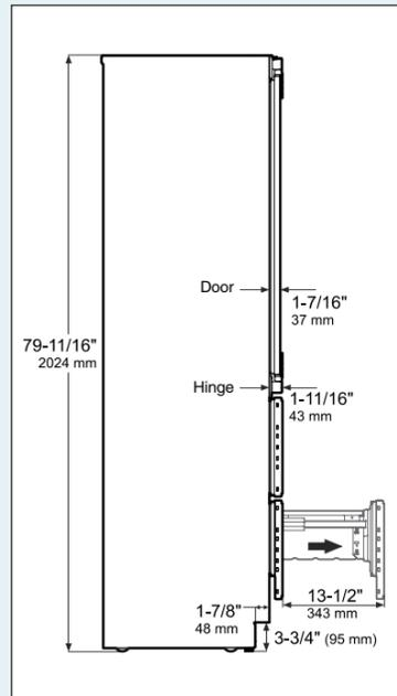
Allow door swing clearance at locations next to a wall. The refrigerator door must open to a minimum of 90° to allow the crispers to open and the shelves to be removed.
