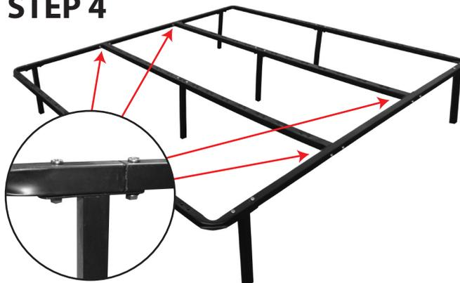
Attach the center supports from Step 3 to the frame from Step 2 using two screws (Part H), two washers (Part J) and two nuts (Part I) for each connection point. Tighten using hex key (Part K) and wrench (Part L).
