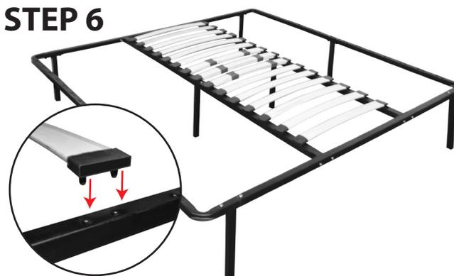
Attach slats to the center section of the frame by pressing the pegs into the holes. Double slats are installed in the middle.
