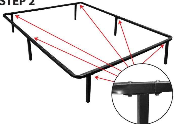
Attach outer six legs (Part E) to the frame using two screws (Part H), two washers (Part J) and two nuts (Part I) per leg. Tighten using hex key (Part K) and wrench (Part L).
