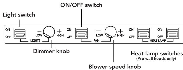
**ON/OFF switch**—Starts and stops the blower. When turned on the blower will operate at the previous setting of the speed control.
