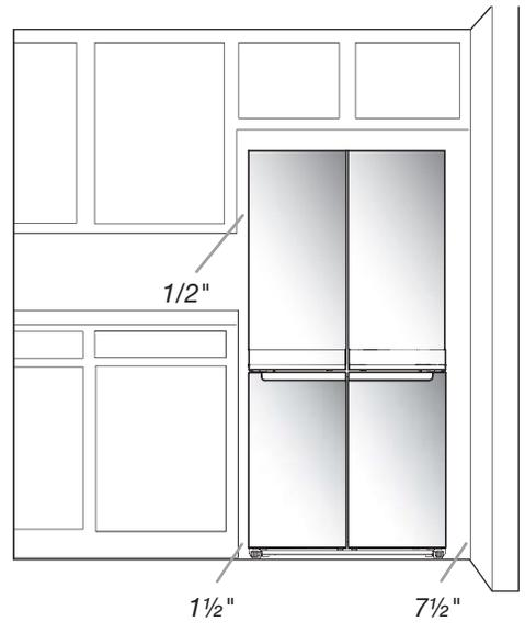
To ensure proper ventilation for your refrigerator, allow for a 1/2" space on each side and at the top. Allow for a 1.97" space behind the refrigerator. If your refrigerator has an ice maker, allow extra space at the back for the water line connections. When installing your refrigerator next to a fixed wall, leave a 3.74" minimum space between the refrigerator and wall to allow the door to swing open.
