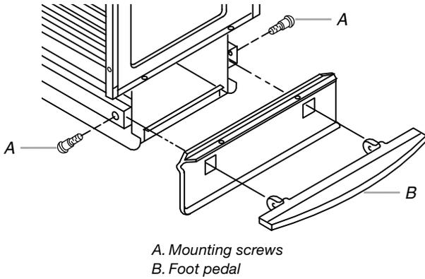
2. Remove mounting screws attaching the toe guard to the compactor. Remove toe guard.
