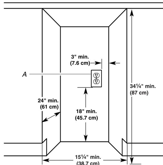
A. Grounded electrical outlet must be a minimum of 3" (7.6 cm) away from surrounding cabinets or nearby walls as shown. It can be placed either to the left or the right side of the product.
