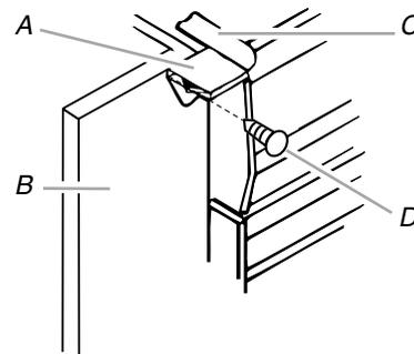
11. Grasp sides of compactor drawer and place bottom of drawer into tracks.
