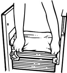
2. Lock bag in place by pulling the 4 prepunched holes over the bag retainer buttons. Holes will expand over the buttons without damaging the bag.
