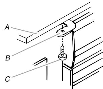
**NOTE:** If retaining brackets cannot be attached to the underside of countertop, attach mounting clips (provided in conversion kit) to retaining brackets. Fasten compactor to kitchen cabinet face with mounting screws through the mounting clips.
