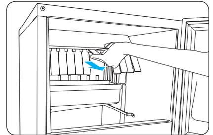
3. Slightly lift the ice slide to remove it.
