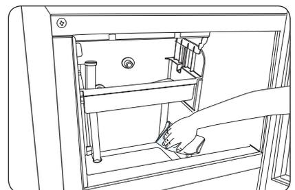
\* Press the switch to set it to (WASH) when cleaning the product; this will repeat the process of supplying water for about 2 minutes and operating the circulation pump 3 times, enabling easier cleaning.
