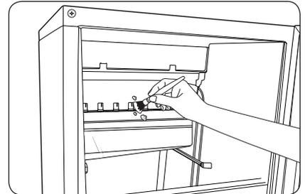
6. Lift the drain connection inside the vessel sheet (water tank), clean it, and drain the water.
