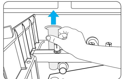
\* The drain connection must be re-assembled in the correct position after cleaning or it will continue to drain and be unable to make ice.
