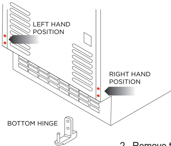
2. Remove the two (2) screws that hold the Bottom Hinge in place. Remove the two (2) corresponding screws on the left hand side. Install the Bottom Hinge in the left hand position and install the remaining two (2) screws into the holes on the right hand side.
