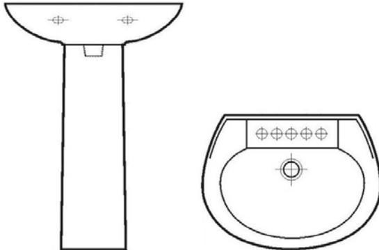
**Be sure to re-inforce wall before installation. We recommend a 2"x12" securely fastened to wall studs at the required height for your installation.**
