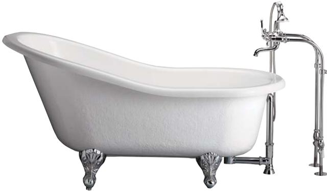
Our acrylic soaker tubs are a fiberglass re-inforced polyester, finished inside with a durable sheet of acrylic. The rough fiber glass exterior is coated with an epoxy paint in either white or bisque to match the interior.
