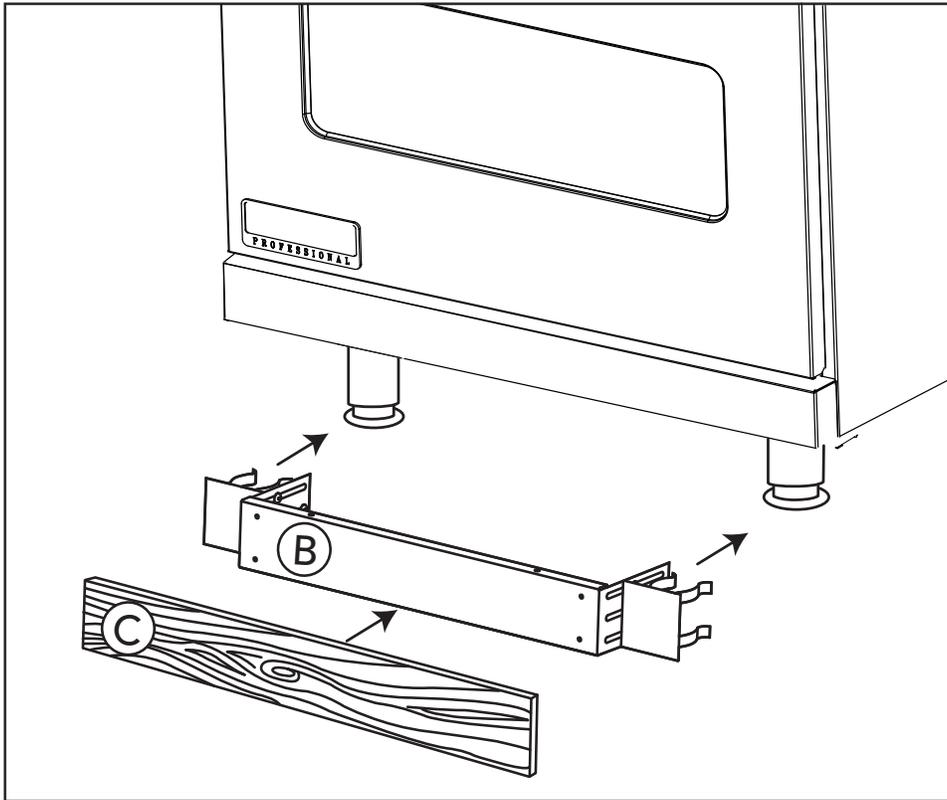
**Important Note:** The range must be installed as specified in the range installation guide for proper airflow when using the custom curb base.
