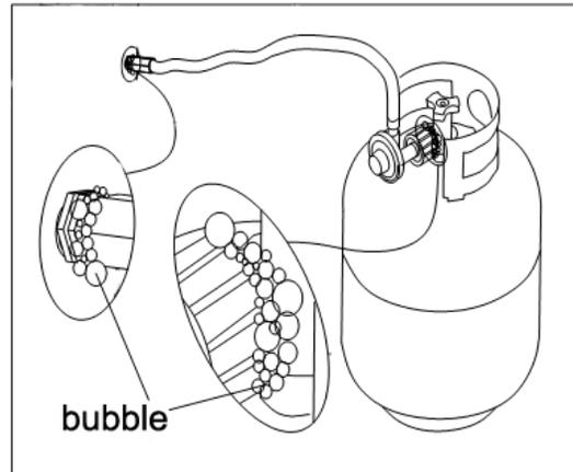
**NOTE:** When leak testing this appliance, make sure to test and tighten all loose connections, including the side burner. A slight leak in the system can result in a low flame, or a hazardous condition.
