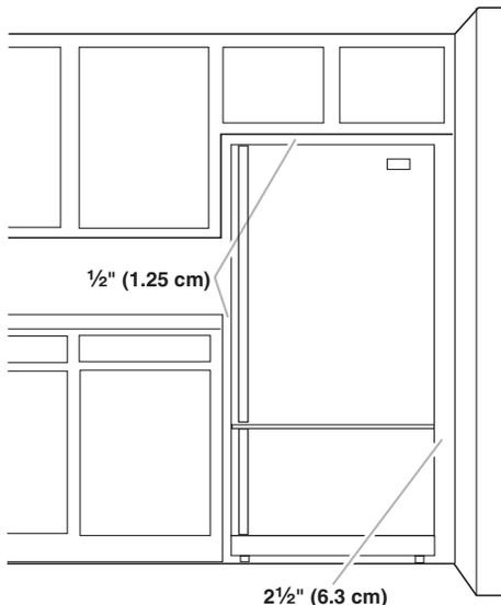
To ensure proper ventilation for your refrigerator, allow for a ½" (1.25 cm) space on each side and at the top. Allow at least 1" (2.54 cm) between back of cabinet and the wall. If your refrigerator has an ice maker, make sure you leave some extra space at the back for the water line connections.
