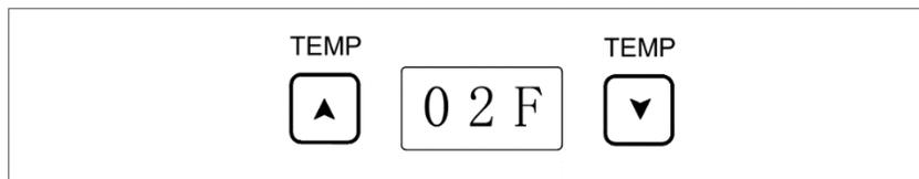
The control panel includes a display that shows the current interior air temperature of the minibar. To change the display between Fahrenheit and Celsius, hold the ▼ button for five seconds.
