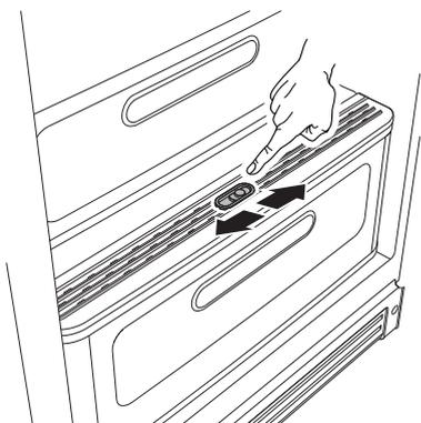
Can be used to adjust the humidity level in the fruit and vegetable drawer. Slide the regulator horizontally to open or close the passage of air through the slots.
