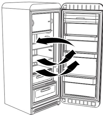
The inner ventilation system cools food more rapidly and keeps refrigeration homogeneous inside the appliance.
