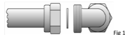
**Warning:** on the cooking top, it is forbidden to carry out the gas connection by means of the rubber flexible pipe fixed onto the rubber hose, as it is not possible to inspect the pipe.
