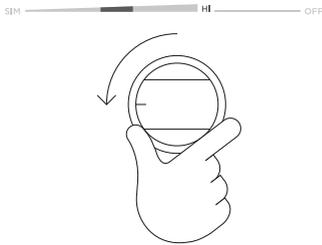
When the burner is lit, turn the dial to any setting between **HI** (high) and **SIM** (simmer).
