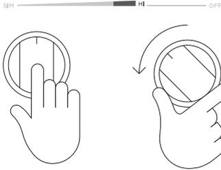
Push the dial in and turn counterclockwise to **HI**. Hold the dial at **HI** before turning to a flame setting.
