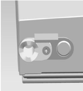
8. Install the door on the refrigerator.
