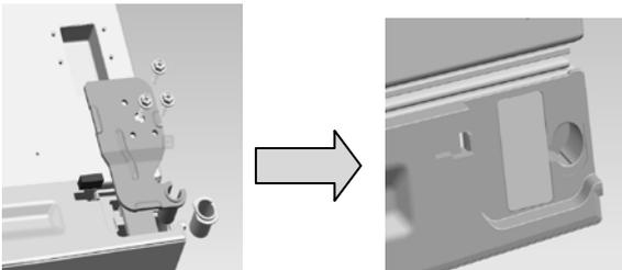
3. Screw off the three bolts fixing the top box cover on the left side, remove the box cover, take the wire harness out of the hole, and transfer the door shaft sleeve from right
