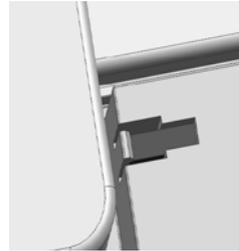
12. Remove the help handle cover, screw off the handle screws, and dismantle the handle, as illustrated by the figure:
