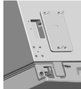
4. Lift up the refrigerator door by 1.97in to remove it.
